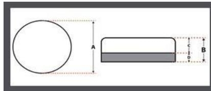
\*Material: Chromium Molybdenum with a mild steel backing 700 bhn
